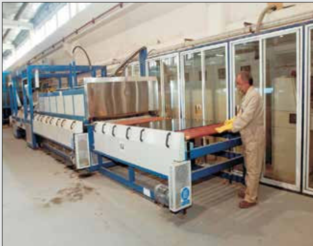
Tempering Line with Forced Convection
