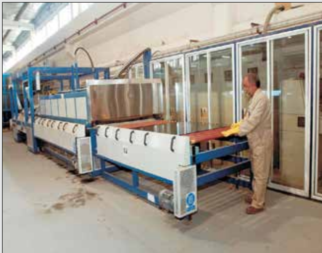
Tempering Line with Forced Convection
